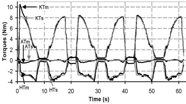
Fig. 5 Torques setpoints for Hip, Knee and Ankle: HTs, KTs, ATs, and Torques measured: HTm, KTm, ATm.
