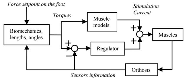
Fig. 4 Functional electrical stimulation control diagram using models of the different stimulated muscles and an orthosis.
