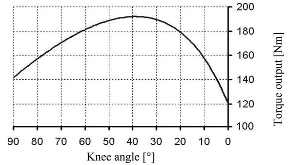
Fig. 3 Torque output of the knee joint regarding the knee angle with a constant motor torque.
