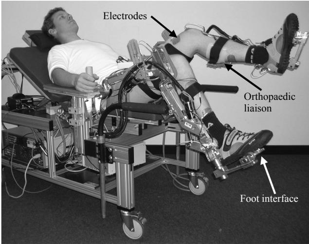
Fig. 1 MotionMaker™ prototype with an uninjured subject.
