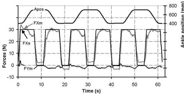
Fig. 6 Horizontal force setpoint (FXs) and measured (FXm), vertical force measured (FYm) during 3 horizontal movements of the ankle (Apos).
