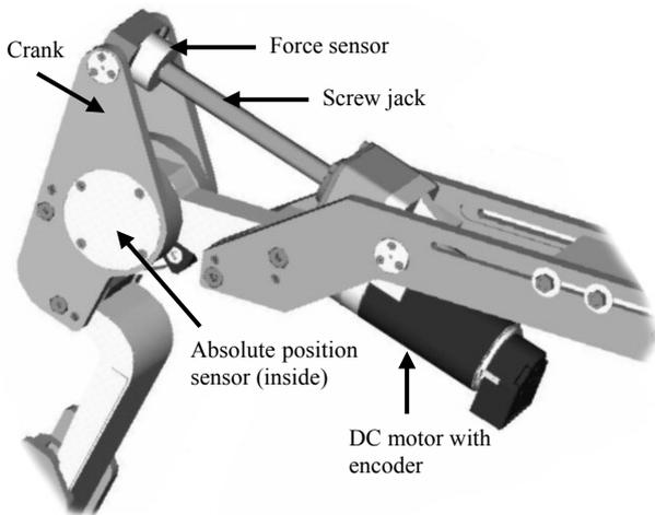
Fig. 2 Detail of the knee joint. Crank and jack architecture with absolute and relative position sensors and force sensor.
