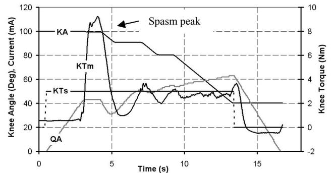
Fig. 7 Spasm management with an injured SCI subject during a closed-loop FES knee extension with a knee orthosis. KA: Knee Angle, KTm: Knee Torque measured, KTs: Knee Torque setpoint, QA: Quadriceps current Amplitude.
