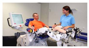
The position and torque sensors, integrated into the orthoses allow to adapt the electrical stimulation and the action of the motors continuously so as to produce exactly the pre-programmed movement and the required muscle force.
