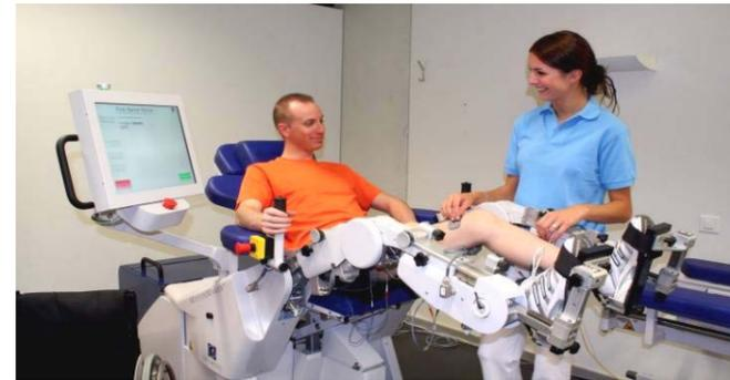
The position and torque sensors, integrated into the orthoses allow to adapt the electrical stimulation and the action of the motors continuously so as to produce exactly the **pre-programmed movement and the required muscle force.**
